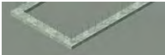
Strip footing with vertical rebar in place.
